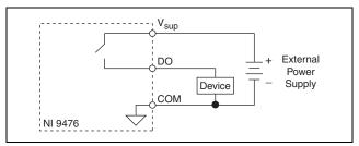
Figure 2. Connecting a Device to the NI 9476
